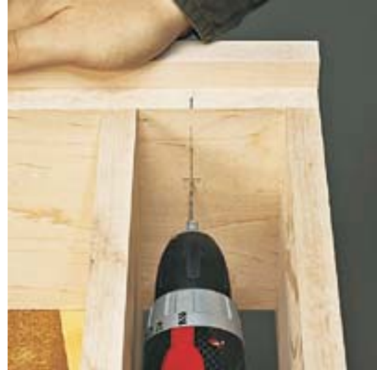
FIGURE 2 Hold the pivoting arm in position and drill a \frac{1}{16} "-diameter hole through the inside of the case and just into the pivoting arm (not all the way through it). This will provide perfectly aligned drilling locations on both pieces.
