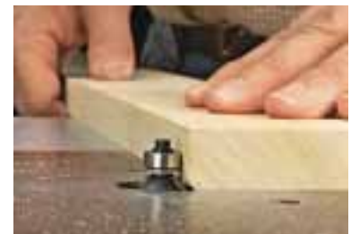
1] After ripping one edge of a long board straight, rout a 1/8" roundover along the edge.
