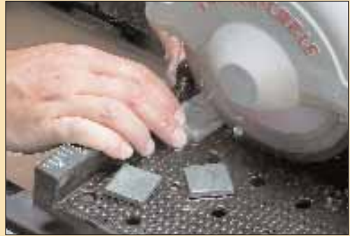
▲ A "wet wheel" tile saw makes quick work of cutting the 3" tile into four pieces. Be sure to keep your fingers back.
